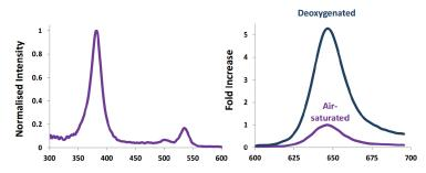
**Figure 1.** Excitation and Emission spectrums of Phosphorescent Oxygen Probe Left panel: shows normalized excitation spectrum of Phosphorescent Oxygen Probe, with emission at 650 nm. Excitation maxima are observed at 380 or 532 nm. Right panel: shows emission spectrum of Phosphorescent Oxygen Probe in oxygenated (purple line) and deoxygenated (black line) conditions with excitation at 380 nm. Under the conditions of measurement, signal increased 5-fold on deoxygenation.
