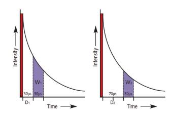
Figure 2. Illustration of ratiometric TR-F measurement
