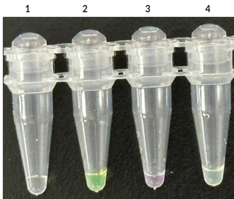
Figure 6. Protein expression using the CFPS ( E. coli ) Kit. Reactions were conducted at 37°C for 3 hours with vigorous shaking. 1: Negative control; 2: sfGFP Positive Control; 3: mCherry; and 4: eGFP
