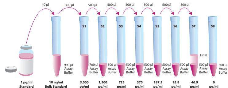
Figure 2. Preparation of the CRP standards
